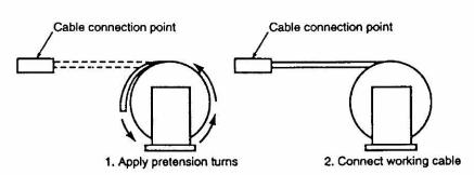
Number of pretension turns depends on application and desired tension. A minimum of 2 set up turns is needed for most applications. Additional tension may be added by repeating above process. After tension is set, connect cable free end. Failure to pretension reel may result in insufficient tension to retract and may shorten spring life.
